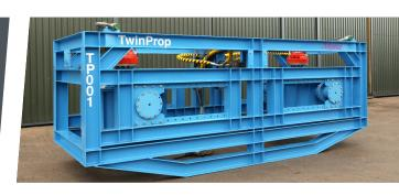
The TwinProp subsea excavation system is the next generation, state-of-the-art development of the widely proven mass flow excavation technique. Counter-rotating propellers are used to produce two high volume columns to rapidly excavate the seabed.
